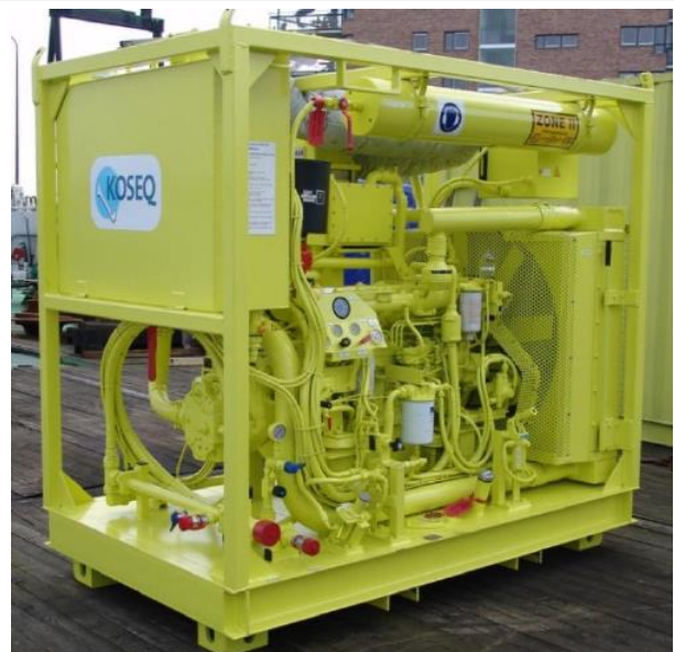
Fig.9 Koseq Hydraulic Power Pack
