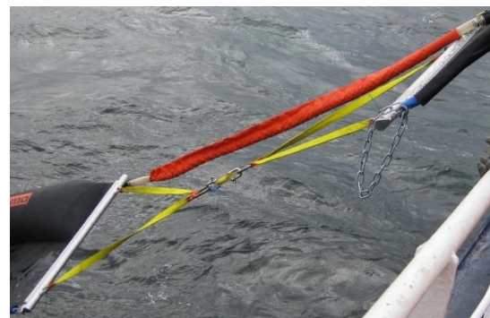
Fig.14 Cross-bridle for open-U
