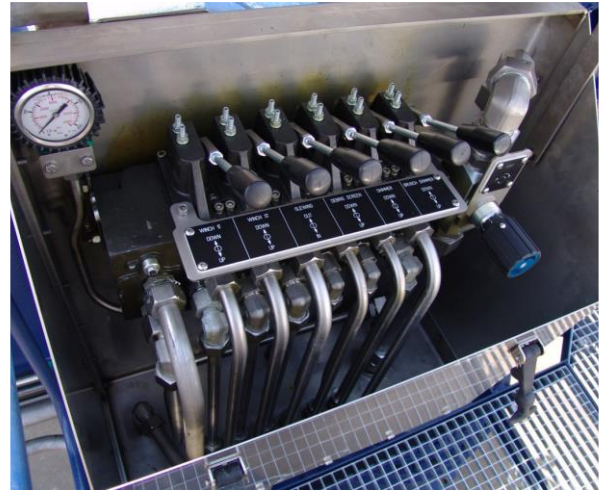
Fig.8 Hydraulic Control Desk
